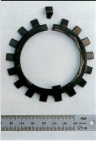
EXTERNAL VIEW OF DAMAGED AND DETACHED WASHER (SAMPLE No.2)
